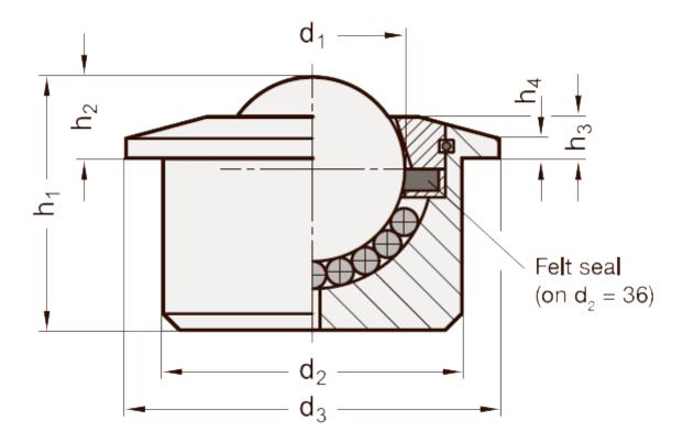
$$\begin{array}{lll} d1 & = 60 \\ d2 + / -0.08 & = 100 \\ d3 & = 117 \\ h1 + / -0.3 & = 77.5 \\ h2 + / -0.3 & = 30 \\ h3 + / -0.3 & = 15 \\ h4 & = 10 \\ Max load (N) = 10000 \end{array}$$
